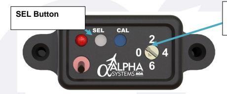
Rotary Switch in Setting Number 1 for Zero Offset Calibration
