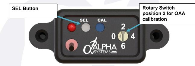
**Note:** If the AOA system indicates a bad set-point, note the display indications at the time of the button push and return to the airport. Make the necessary angle adjustments, relative to the direction of the error code, to the AOA probe. Adjust the probe in 5 degree increments. When the AOA probe angle adjustments have been made, perform the entire in-flight calibration procedure outlined in this section until you are successful.
